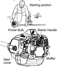
NOTE: The throttle lock-out is designed to prevent unintentional use of the throttle trigger. The lock-out must be pressed with the palm of your hand as you grip the throttle handle before the trigger can be used. DO NOT squeeze the throttle trigger until the engine has started and runs.
